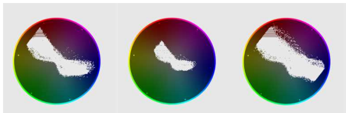
Figure 2. (a) Vectorscope of original image, (b) vectorscope of image with reduced saturation, (c) vectorscope of image with increased saturation
